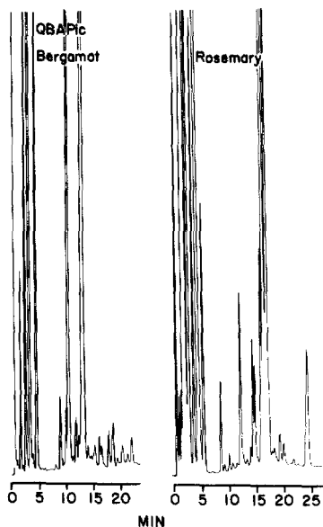
Fig. 10. Separation of oils of bergamot and rosemary on a 2 m \times 2 mm I.D. column of 10% (w/w) tetra- n -butylammonium picrate (QBAPic) on Chromosorb W-AW (100–120 mesh) with a nitrogen carrier gas flow-rate of 20 ml/min. The column was temperature programmed from 90 to 150°C at 3°C/min for oil of bergamot and 5°C/min for oil of rosemary.
